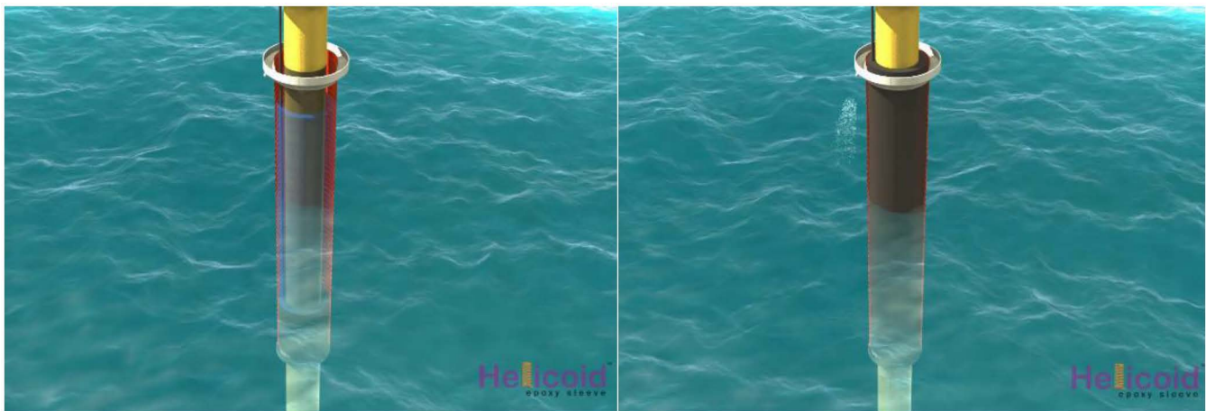
Figure 12—Injection of Epoxy Grout via Tremie Method
