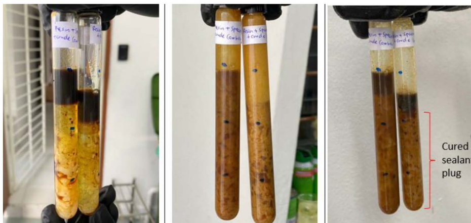
Figure 12(c)—From left to right, mixture of sealant spacer, neat resin sealant and crude oil, followed by shaken process and sealant plug condition after 24 hours curing process in 40° Celsius water bath.
