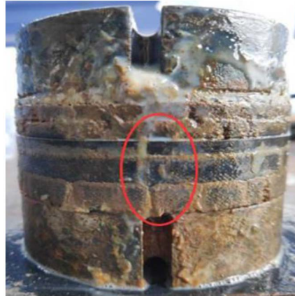
Figure 9(c)—Activated sealant in solid form observed across the leak path created competent seal.
