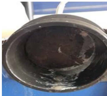
Figure 7(c)—No excessive sealant was squeezed outside of the injection cavity.
