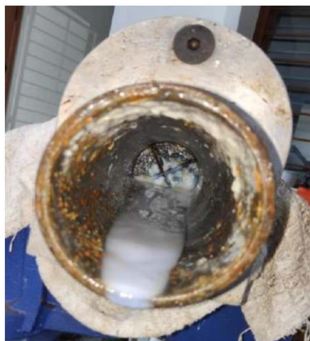
Figure 9(b)—Inactivated sealant in liquid form remain after depressurise pressure chamber for leak sealing simulation.
