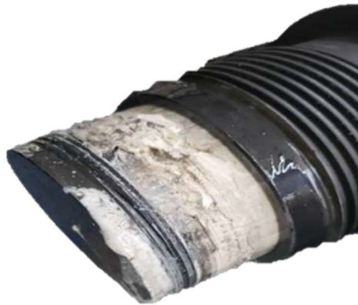
Figure 7(b)—A competent seal was observed when removing the simulated injection cavity.
