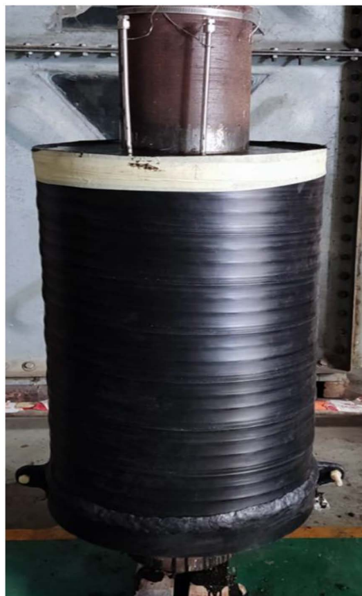
Figure 8(b)—Conductor leak test fixture condition after tubing diverter installation and cured epoxy grout.
